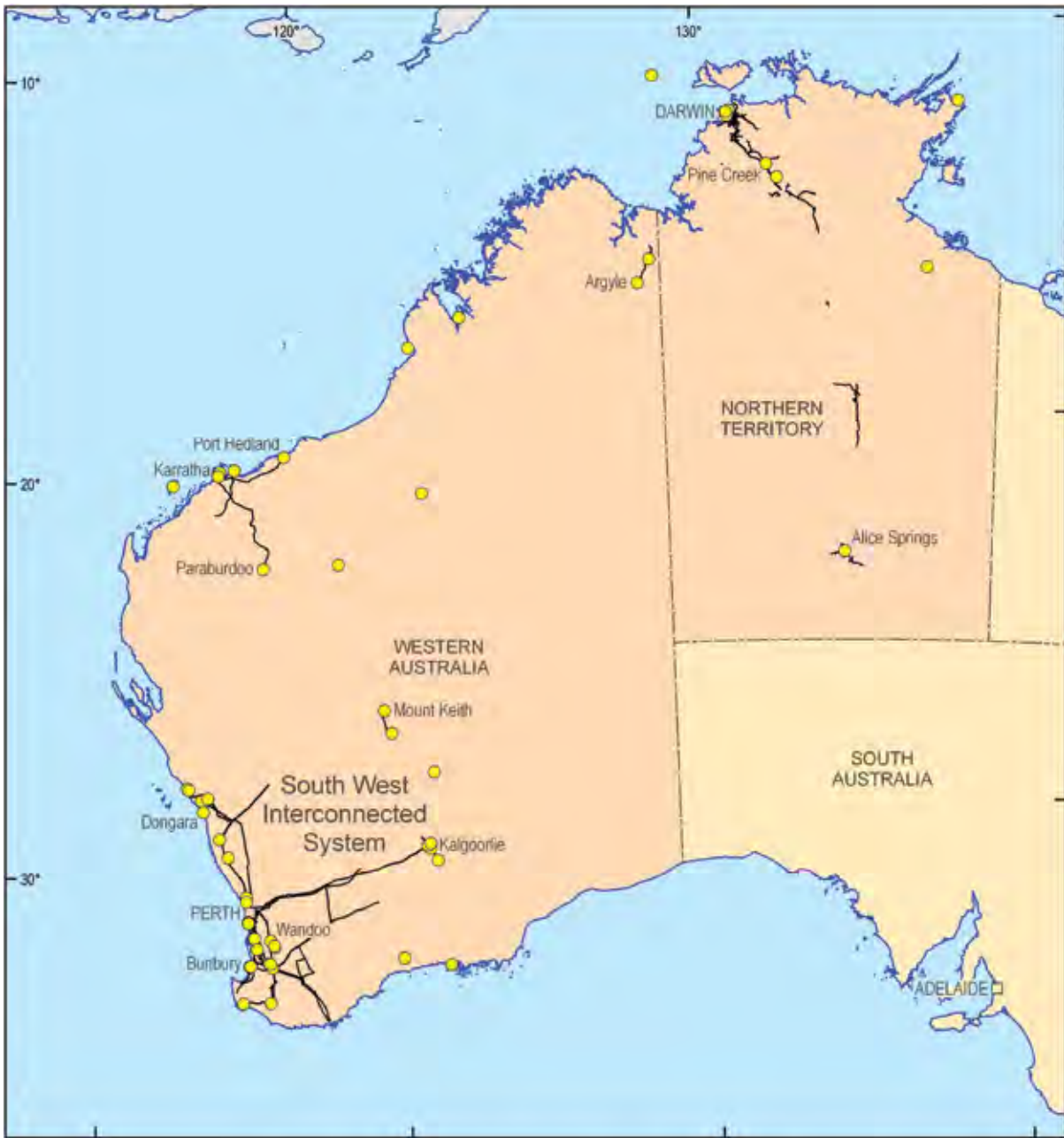
Figure 4.2: Northern and Western Australian electricity transmission systems
